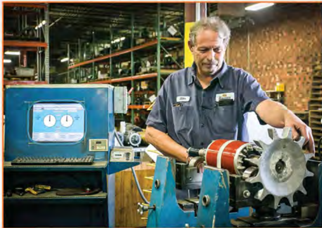
Shaft balancing to military specifications
